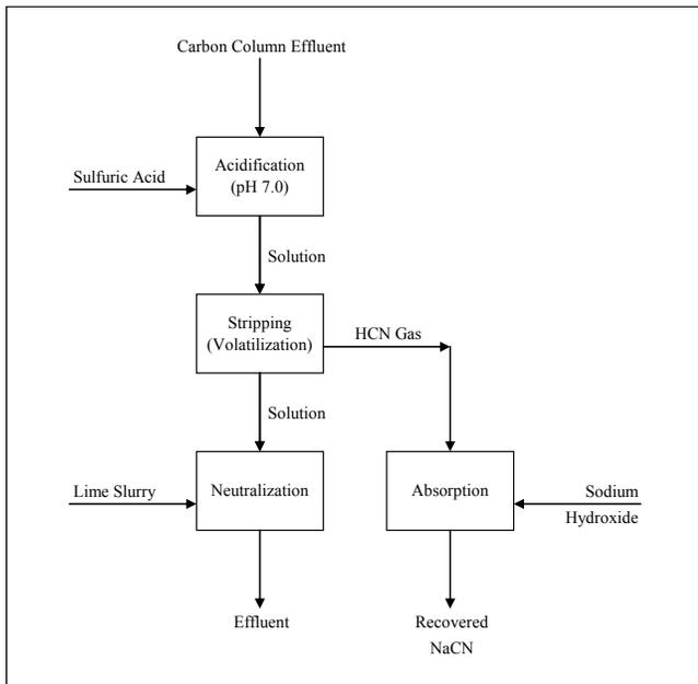
**Figure 3.** Cyanide Recovery Flow Diagram
